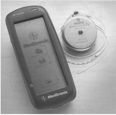
Fig. 1. The SynchroMed II pump and handheld telemetry programmer. Photo provided courtesy of Medtronic Inc
