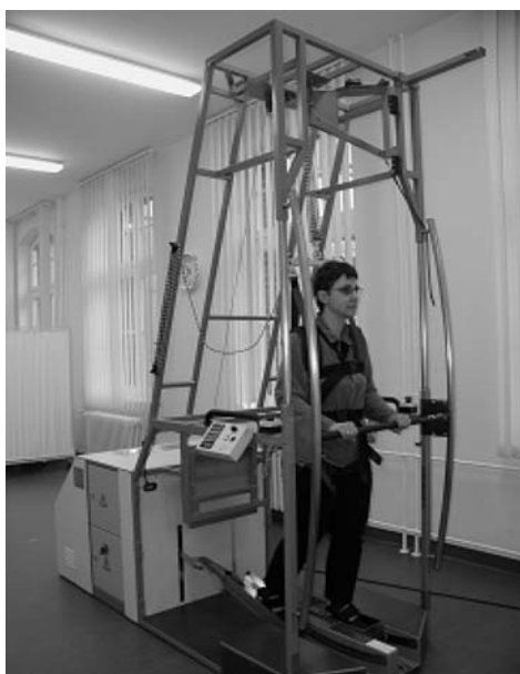
Fig. 3. Advanced Gait Trainer ® . The robot that moves feet mimicking life-like movements. The system provides controlled body-weight support. The robot is available from Company Reha Stim, Berlin, Germany
