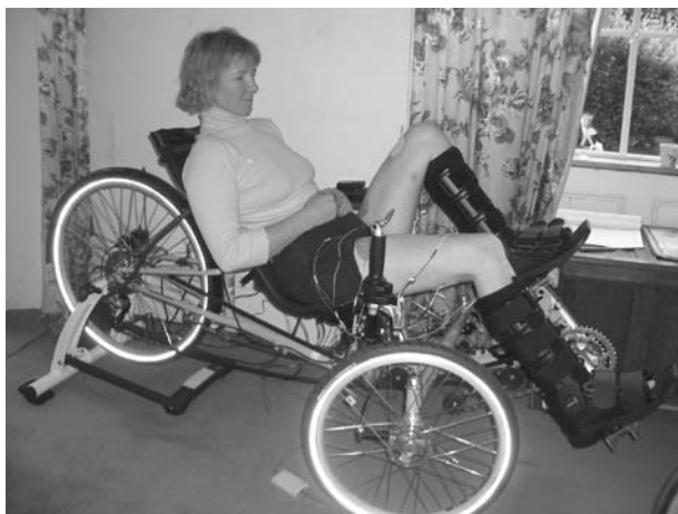
Fig. 1. FES exercise at home with tricycle on friction roller ("trainer"). The ankle orthoses, throttle, and electrodes on quadriceps and hamstring muscles can be seen. The tricycle was designed for mobile use and has standard gears and brakes. Transfer from a wheelchair is not difficult because the seats are at similar height and an upstanding handle can be temporarily detached from the handle bar
